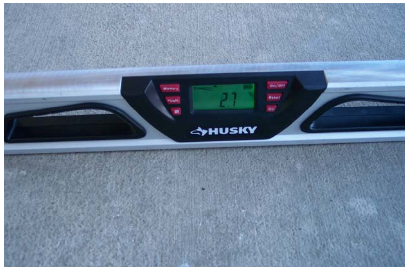
K4. Rear Exit POT Slope at Door
